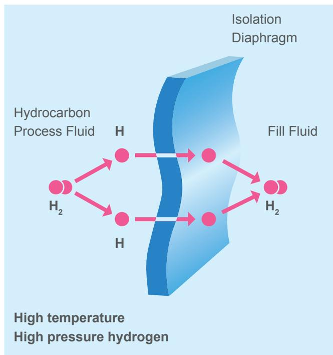
$H^+$  ions permeate the diaphragm and re-unite behind the diaphragm.
