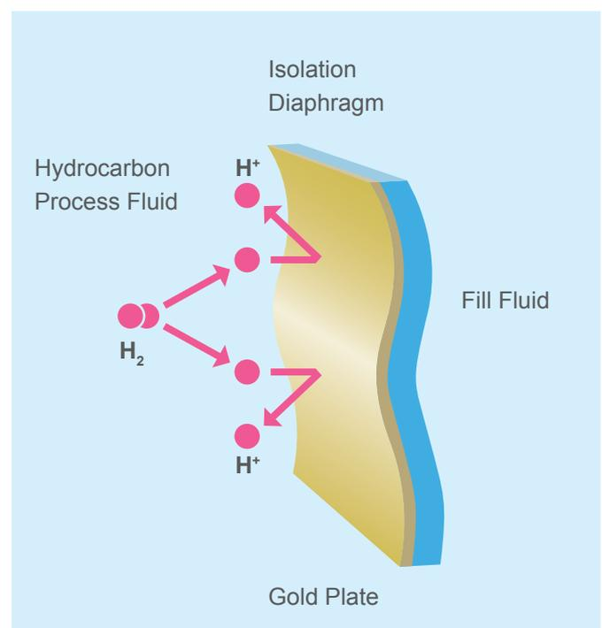
A layer of gold coating protects the  $H^+$  ions from permeation through the diaphragm.
